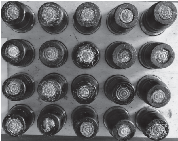
Photo No. 4 – swollen and salt efflorescence on the pyrotechnic mixture of tracers from anti-aircraft ammunition (own source)
