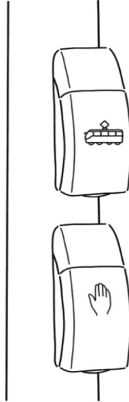
Fig. 3. Diagram of the placement of the “tram button” on the traffic signal pole
