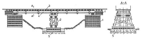
Fig. 3. Provisional bridge reconstruction (Cholewo & Sznurowski, 1970; Miklin & Sawicki, 1993): 1 – railway sleeper cages forming the bridge abutments, 2 – provisional support in the form of a wooden yoke, 3 – railway pavement, 4 – provisional span, 5 – substructure of the intermediate support in place of the destroyed pillar of the fixed bridge
