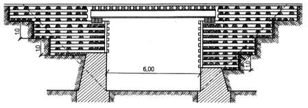
Fig. 4. Provisional reconstruction of a bridge with a span made of I-beams on supports (abutments) made of railway sleepers forming so-called cages (Cholewo & Sznurowski, 1970; Miklin & Sawicki, 1993)
