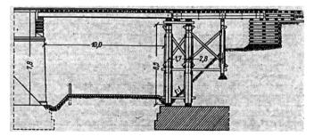
Fig. 5. Provisionally reconstructed viaduct (Cholewo & Sznurowski, 1970): left span made of steel I-sections; right span made of wooden beams; central pillar of frame construction set on the foundation of the destroyed abutment
