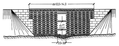
Fig. 2. Filling the opening of a damaged bridge using a structure in the form of 'cages' made of railway sleepers (Cholewo & Sznurowski, 1970; Miklin & Sawicki, 1993)
