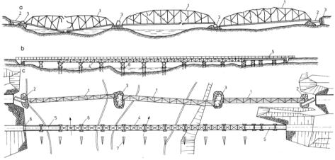
Fig. 11. Bypass bridge (Miklin & Sawicki, 1993): a - side view of the destroyed permanent bridge, b - side view of the temporary (bypass) bridge, c - top view of the destroyed bridge and location of the bypass bridge; 1 - destroyed lattice spans,
