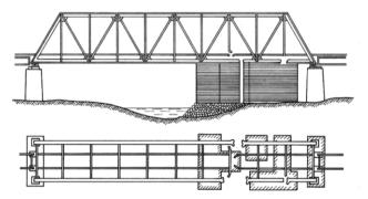
Fig. 10. Method of ad hoc reconstruction of a damaged truss with a bottom ride using additional supports constructed as cages from railway sleepers (Miklin & Sawicki, 1993)
