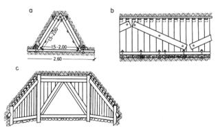
Fig. 1. Provisional culvert with a triangular cross-section made of railway sleepers (Cholewo & Sznurowski, 1970; Miklin & Sawicki, 1993): a – cross-section, b – side wall reinforcement, c – view from the inlet to the culvert
