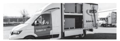
Fig. 3. Double floor in a vehicle with a GVM <3.5 t Source: https://botam.eu/rozwiazania/, access date: 07/03/2022.
